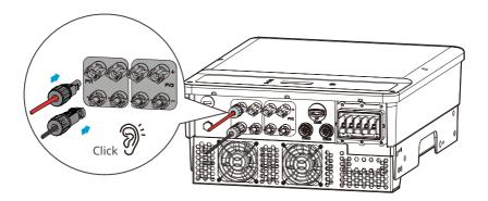
Seal the PV input terminals using waterproof covers when they are not to be used. Otherwise, the ingress protection rating will be influenced.
