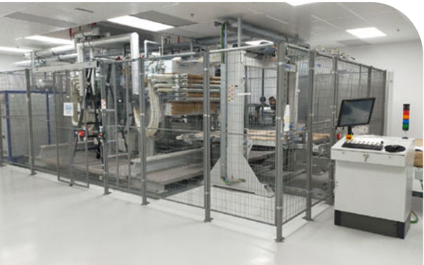
Photovoltaic Module Laminator
