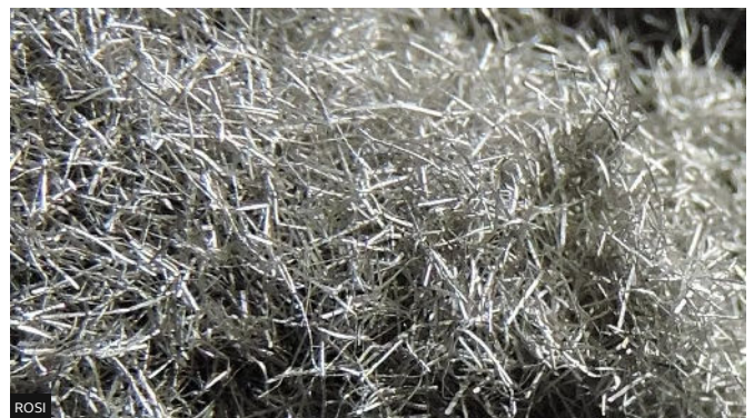
Silver fragments recovered from solar panels, at the ROSI plant in Grenoble
