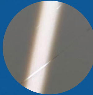
Widespread backsheet cracking PVDF
