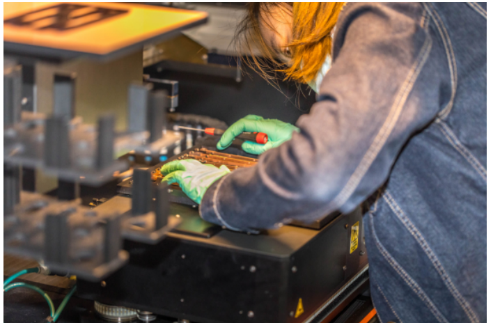
A UNSW researcher measuring the current-voltage characteristics of an industrial TOPCon silicon solar cell. Image from Bram Hoex
