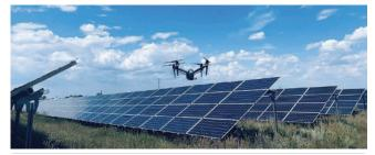
Thermographic surveys by drones can be used to evaluate common module defects Image: Above
