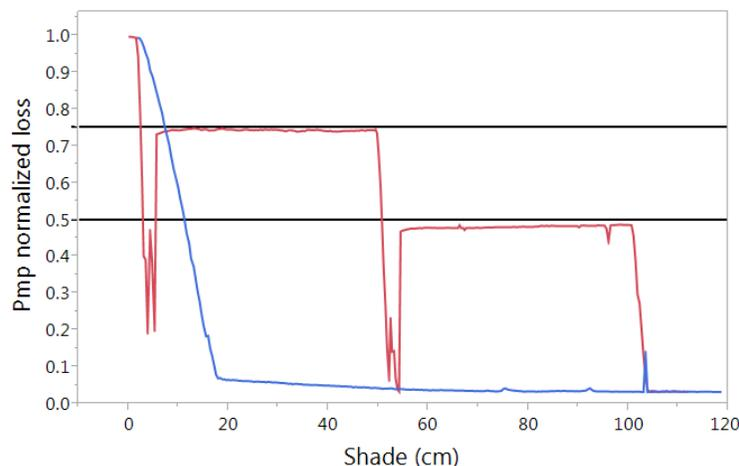
Figure 4.1.2 Normalized loss function in portrait, P-Series (red) and conventional solar panel (blue)
