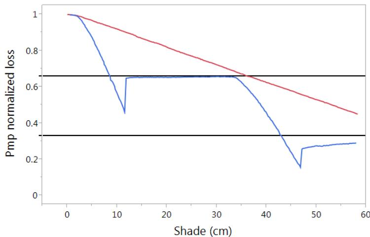
Figure 4.1.1 Normalized loss function in landscape, P-Series (red) and conventional solar panel (blue)
