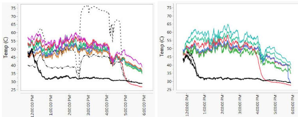
Figure 4.1.5 Module temperature trends for P-Series (left) and conventional solar panel (right) in portrait
