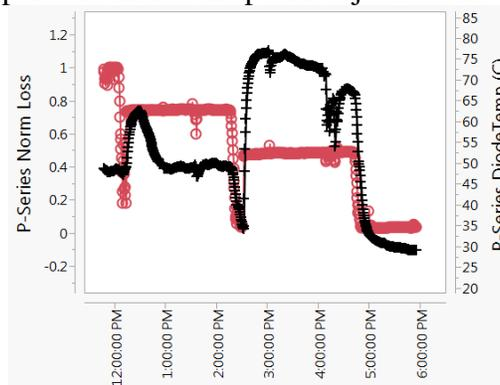
Figure 4.1.6 P-Series loss function (red) and bypass diode temperature (black) in portrait
